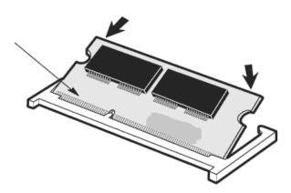
Figure 40. SODIMM Installation – Applying Pressure
